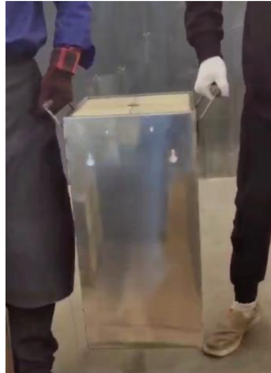
DeNOx catalyst (1 module out of 60)
