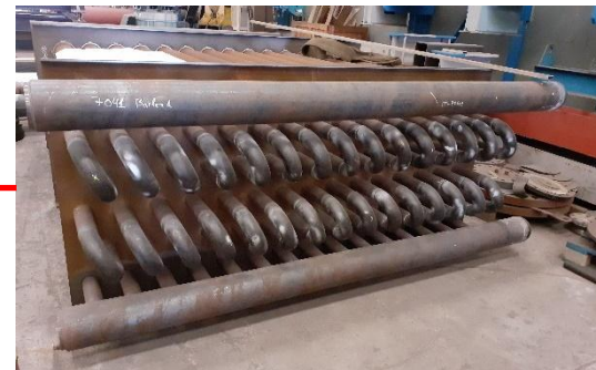
Boiler SA-106 Gr. B
